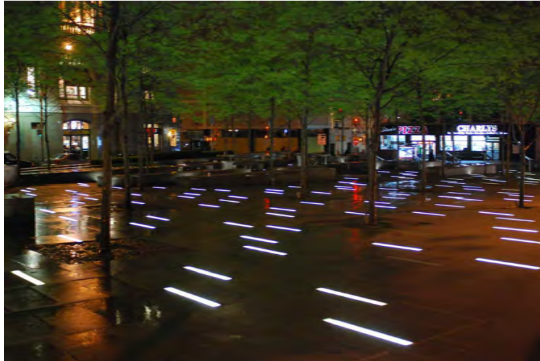
IN-GROUND LED WAY FINDING LIGHTS
